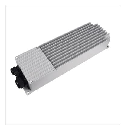
Class I non-insulated, 1800W (600W x 3 channels) output constant current DALI-2 programmable. An IP66 enclosure makes it also suitable for outdoor applications and its electrical characteristics make it suitable for TV broadcasting applications.
