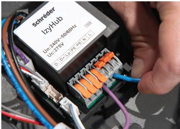
IzyHub is a luminaire electrical connection hub with built-in surge protection. The hub allows easy connection to the end user mains network with no additional tools required.
